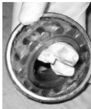
Fig. 21. Grease can easily be packed by hand.
