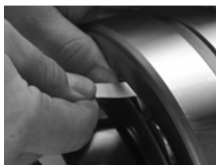
Fig. 14. Measure RIC before installation.
