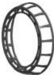
Fig. 3. EJ steel cage.
