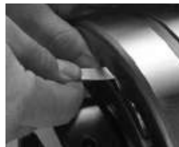
Fig. 18. Measure RIC before installation.
